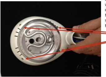
careful not to stretch as there are wires running through. You just need enough remove so you can turn the top upside down to gain access to the screws underneath. Remove these four screws shown below.
